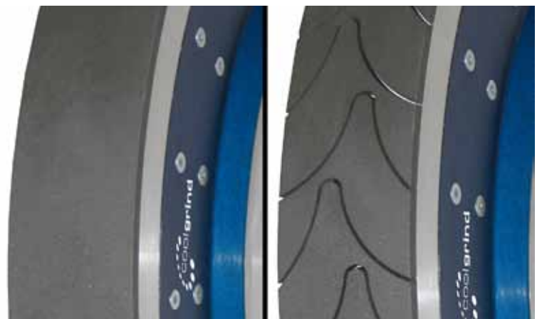
Detailed view: coolgrind-grinding wheel before and after the alteration (picture 3)
